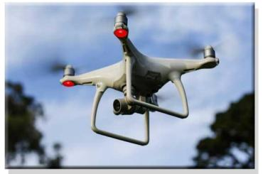
At present, all over the world in the production of engineering surveys are widespread receive UAV (unmanned aerial vehicle) for aerial photography and compilation 3D models of terrain.
